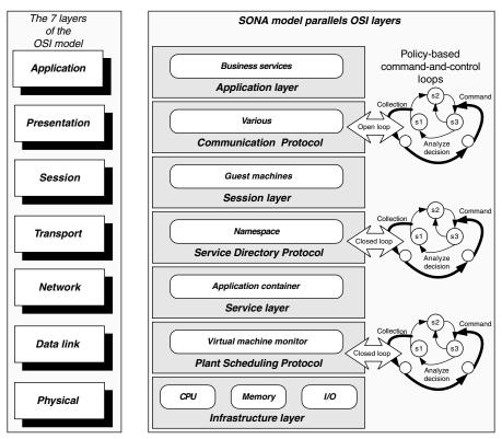
Figure 18.5. SONA layers parallel the OSI seven-layer model.
